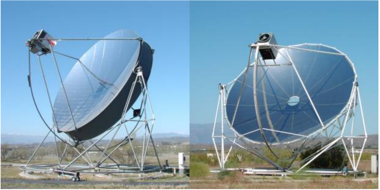
Şekil 3: Çanak–Stirling sistemi [kaynak: https://www.volker-quaschnig.de/articles/fundamentals2/index_e.php ]
